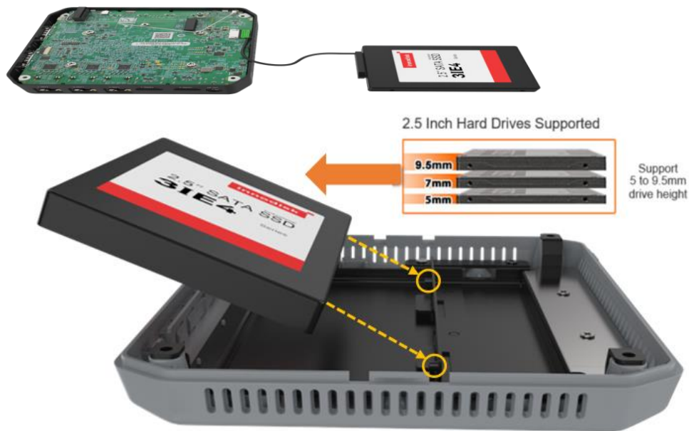
Figure 5-6: Connect the HDD/SSD and Align with the Bracket
