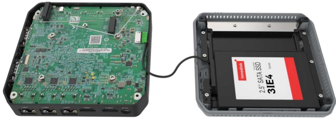
Figure 5-7: Seat the HDD/SSD to the Bracket
