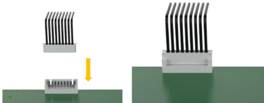
Figure 3-9: RS-232 Cable Installation
