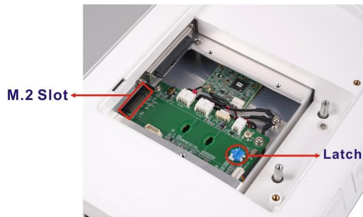
Figure 3-6: M.2 Slot Location
