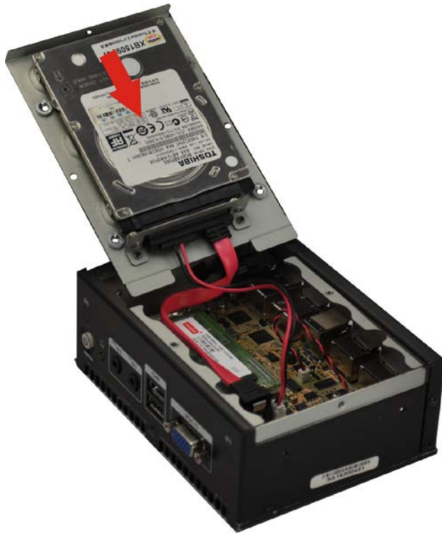
Figure 3-3: Insert the HDD
