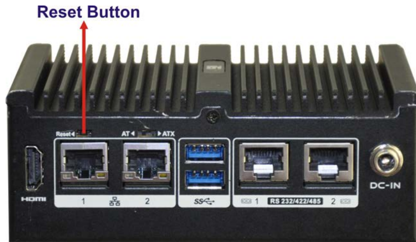
Figure 3-13: Reset Button Location
