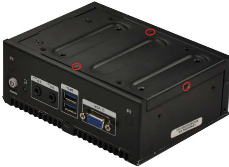
Figure 3-1: Retention Screws Removal
