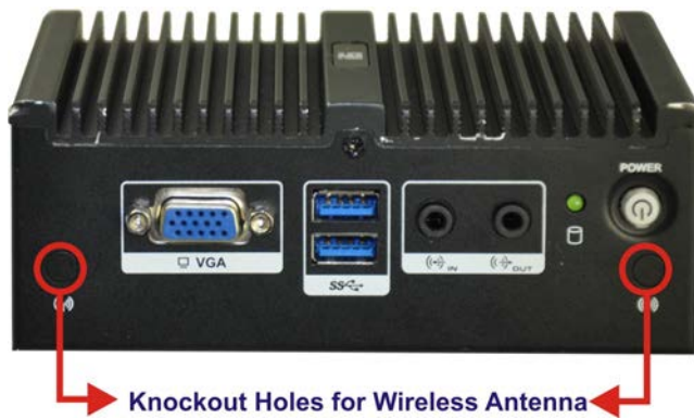
Figure 3-5: Knockout Holes for Wireless Antenna
