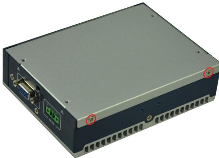
Figure 3-11: Remove the Bottom Panel (ITG-100-AL-E1/S)
