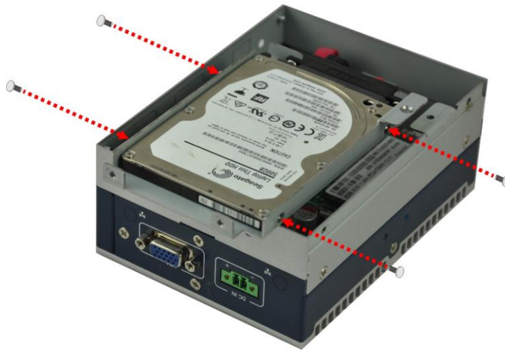
Figure 3-3: Install the HDD
