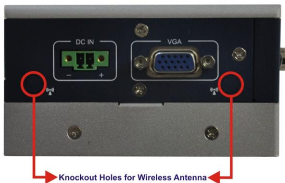
Figure 3-6: Knockout Holes for Wireless Antenna
