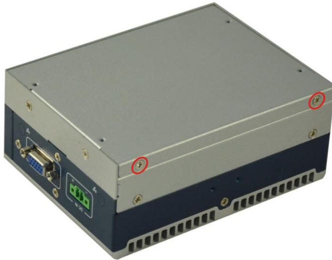
Figure 3-14: Reinstall the Bottom Panel (ITG-100-AL-E1)
