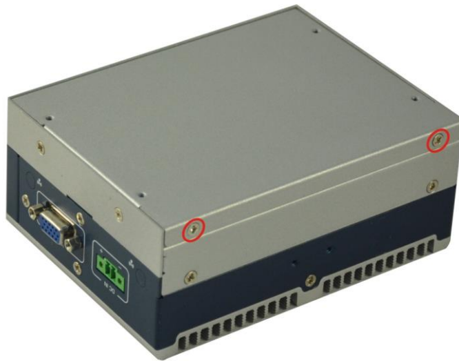
Figure 3-1: Remove the Bottom Panel
