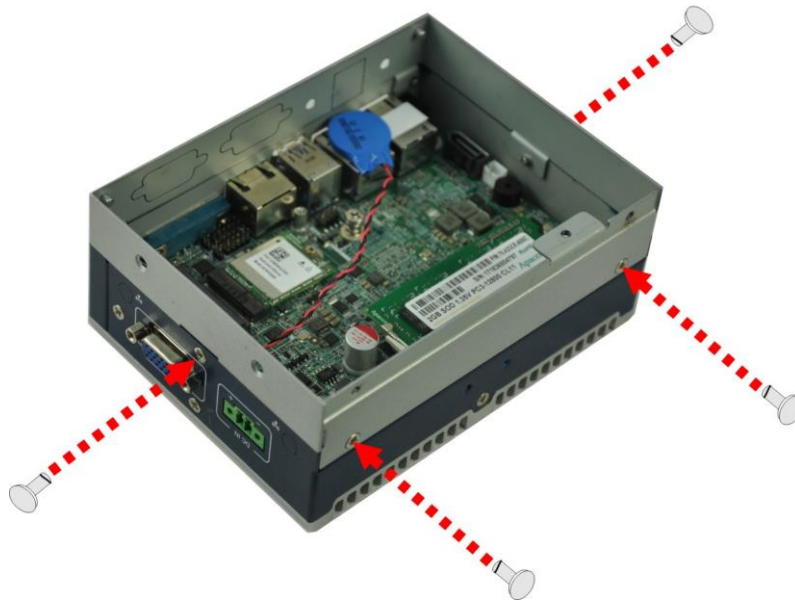
Figure 3-12: Additional Block Layer Installation
