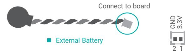
The external lithium ion battery supplies power to the real-time clock and CMOS memory as an auxiliary source of power when the main power is shut off.
