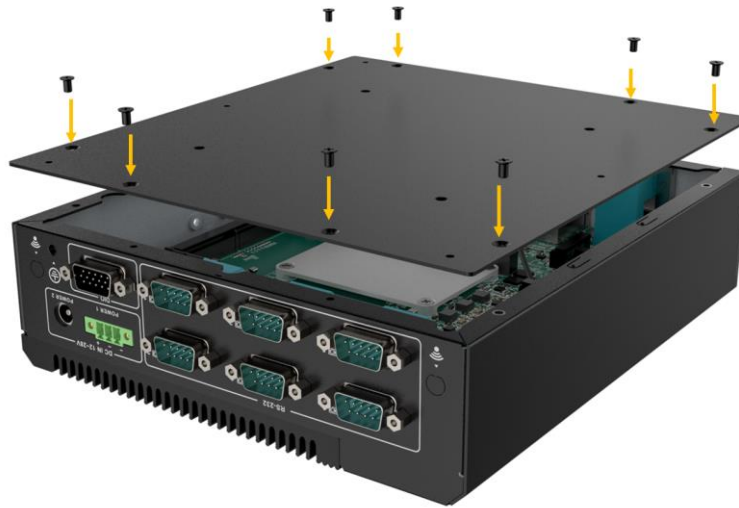
Figure 3-4: Reinstall the bottom cover
