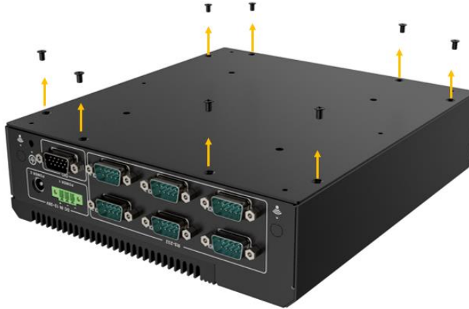
Figure 3-1: Remove Retention Screws (Bottom Panel)
