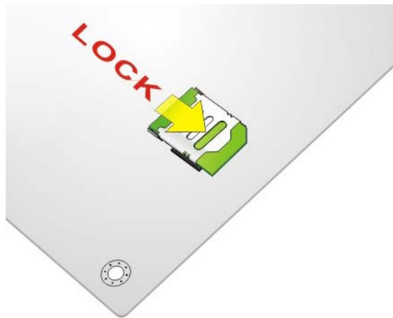
Figure 4-13: Lock SIM Card Slot Cover
