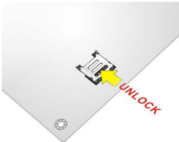
Figure 4-11: Unlock SIM Card Slot Cover
