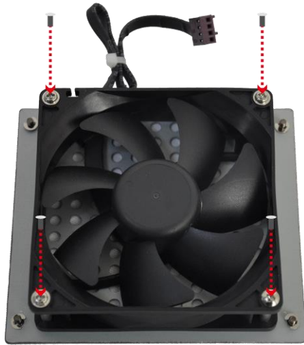
Figure 3-5: System Fan Installation
