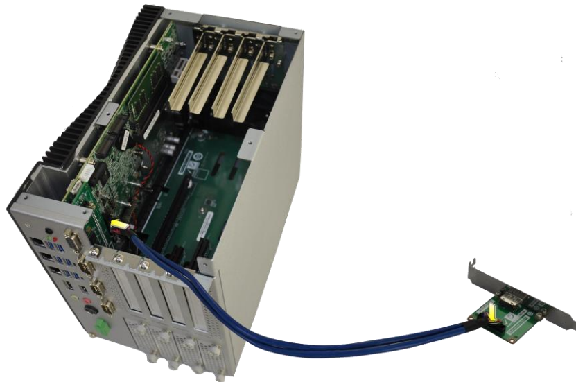
Figure 3-19: iDP Module Installation
