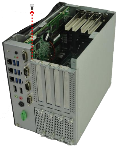
Figure 3-20: Remove Expansion Slot Bracket
