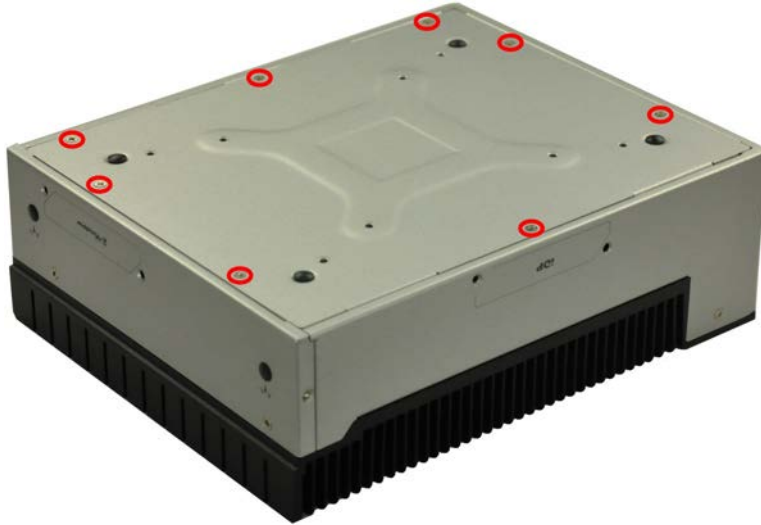
Figure 3-1: Bottom Panel Retention Screws
