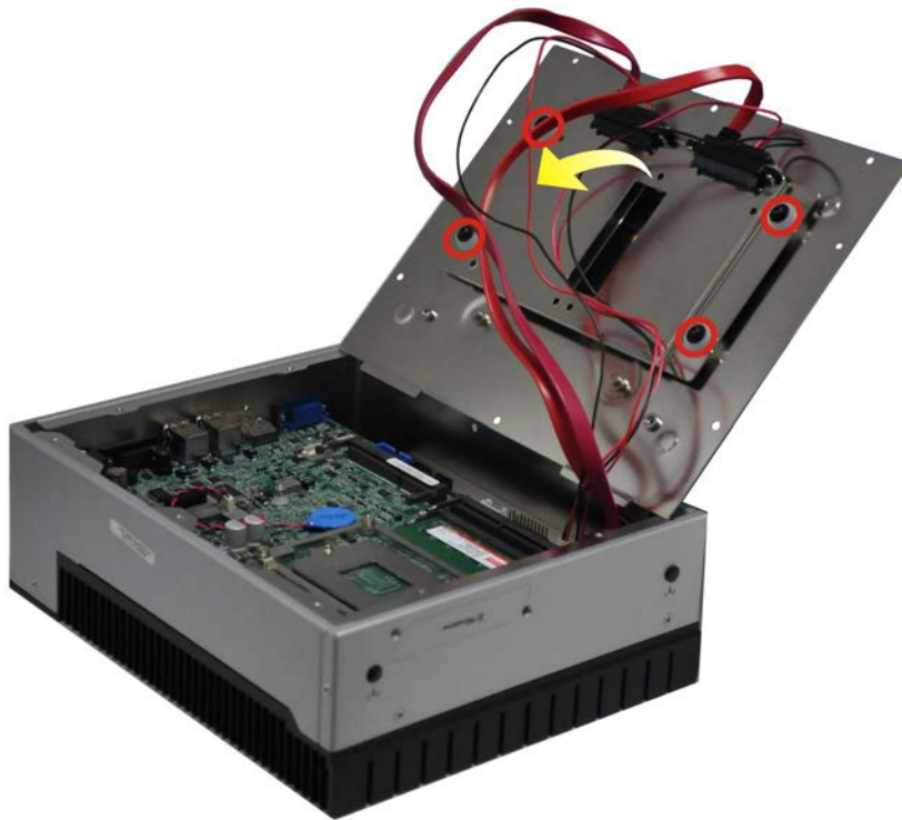
Figure 3-2: HDD Bracket Retention Screws
