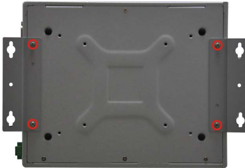
Figure 3-6: Mounting Bracket Retention Screws
