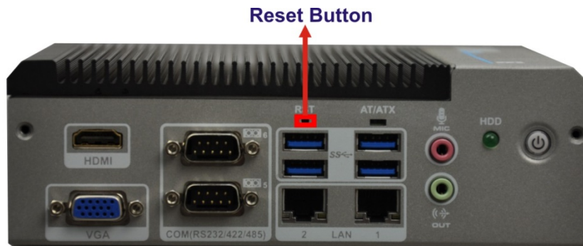
Figure 3-14: Reset Button Location
