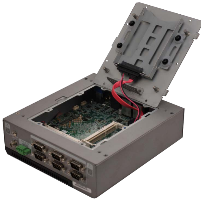
Figure 3-2: HDD Bracket Retention Screws
