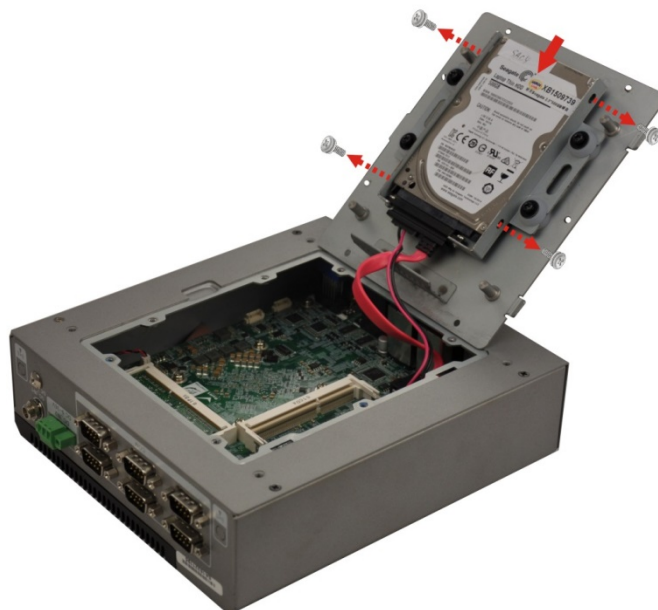
Figure 3-3: Inserting the HDD
