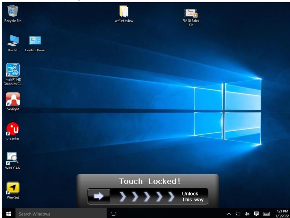
Press F1 and F2 simultaneously one more time to perform unlock touch function, or you can slide the bar to unlock the touch lock.
