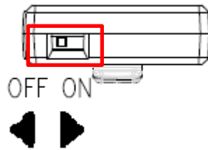
Figure 7: MV type hardware write protect position
