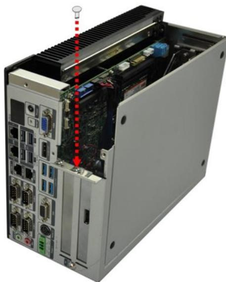
**Figure 3-26: Secure iDP Module to System**
