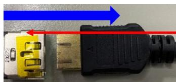
For DP connection, just plug in as normal because the connector size is the same as the DisplayPort cable.
