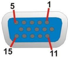
Figure 3-21: VGA Connector
