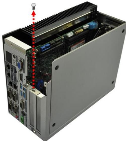
**Figure 3-25: Remove Expansion Slot Bracket**
