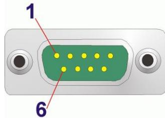
Figure 3-18: DB-9 RS-232/422/485 Serial Port Connector
