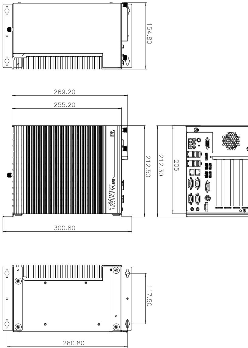
**Figure 1-10: TANK-870-Q170-4 slot Physical Dimensions (millimeters)**
