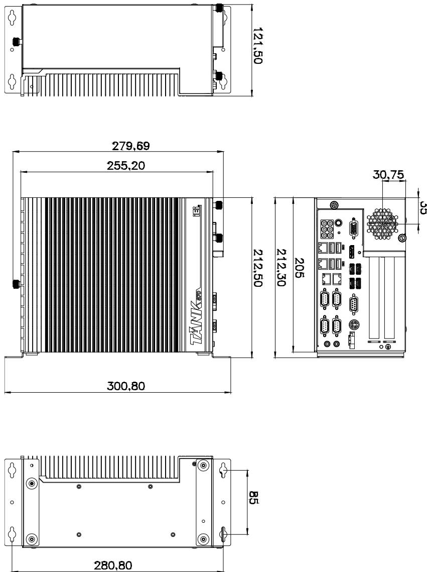
Figure 1-9: TANK-870-Q170-2 slot Physical Dimensions (millimeters)
