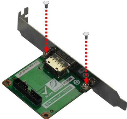
**Figure 3-23: iDP Module with Bracket**
