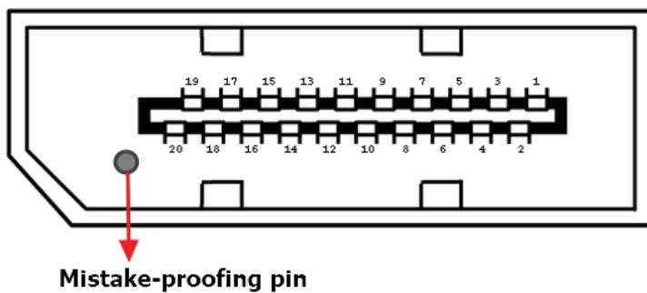
Figure 3-11: DP/HDMI Connector Pinout Locations
