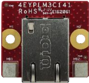
Figure 3: Mounting Hole Daughter Board Picture (EGPL-T102-C1)
