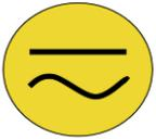
**ALTERNATING CURRENT** This product must be grounded. Use only a grounded AC outlet. Install the additional PE ground wire if the local installation regulations require it. *\*If you do not use a grounded outlet while using the device, you may notice an electrical tingling sensation when the palms of your hands touch the device.*
