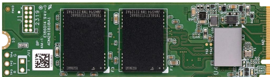
Figure 1: Innodisk M.2 (P80) 3TE4 (type 2280)
