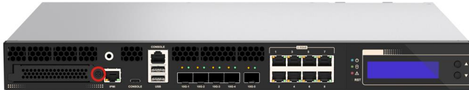
Figure 3-10: OCP 3.0 Slot Cover Screw
