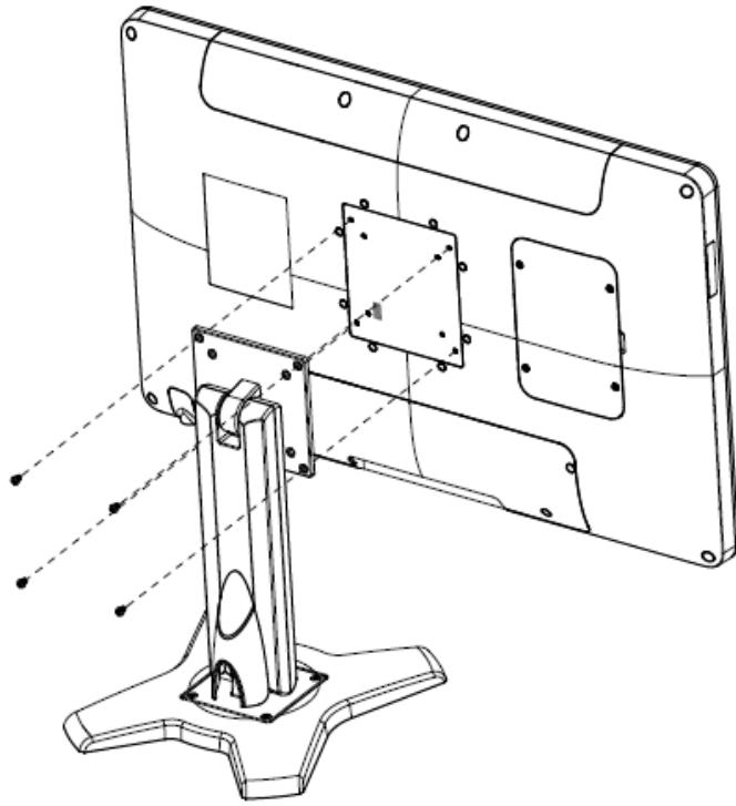
**Step1.** Position VESA Mount on both sides, matching the holes on the system.
