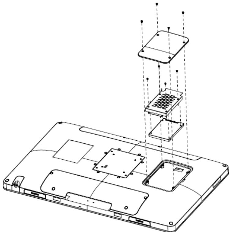
**Step1.** Remove 4 screws to release the chassis cover and remove it.
