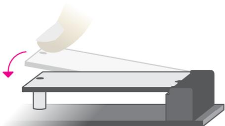
Step 2: Press the end of the card far from the socket down until the gap between the card and the stand-off closes up.
