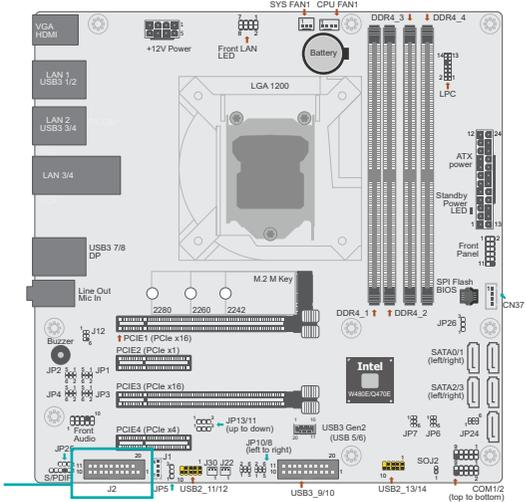
The 16-bit Digital I/O connector provides powering-on function to external devices that are connected to these connectors. The pin functions of the 16-bit digital I/O connector are listed below.
