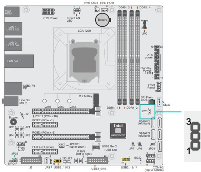
JP26 is used to switch between AT/ATX Mode.
