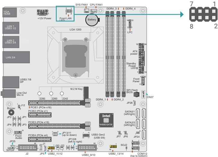
The LAN LED connector is used to detect the connection state of RJ45 LAN ports when the connection is made to an active network via a cable. The pin functions of the LAN LED connector are listed below.
