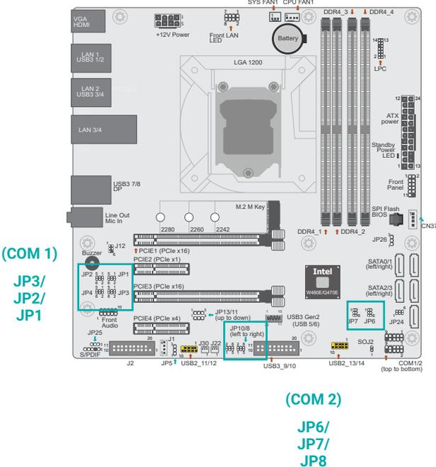
JP1/JP2/JP3 (for COM 1) are used to configure the COM ports to RS232, RS422 (Full Duplex) or RS485. When COM 1 RS232/422/485 is selected, JP1 and JP2 must be set in accordance to JP3. COM 2 uses the same principle applied to the JP6/JP7/JP8.
