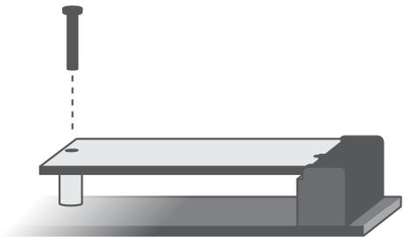
Step 3: Screw tight the card onto the stand-off with a screw driver and a stand-off screw until the gap between the card and the stand-off closes up. The card should be lying parallel to the board when it's correctly mounted.
