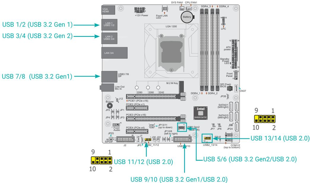
The USB device allows data exchange between your computer and a wide range of simultaneously accessible external Plug and Play peripherals.
