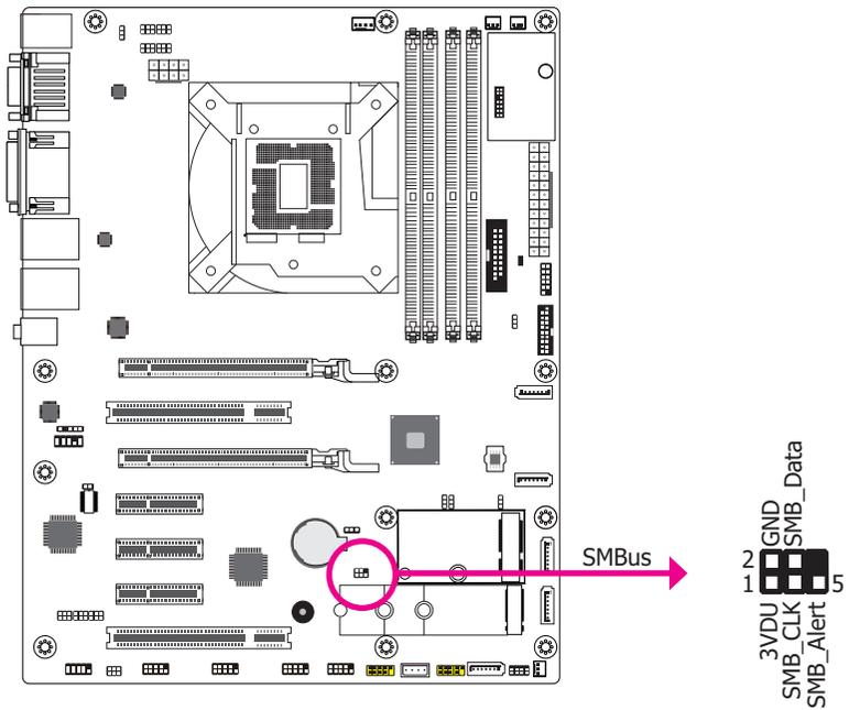
The SMBus (System Management Bus) connector is used to connect SMBus devices. It is a multiple device bus that allows multiple chips to connect to the same bus and enable each one to act as a master by initiating data transfer.
