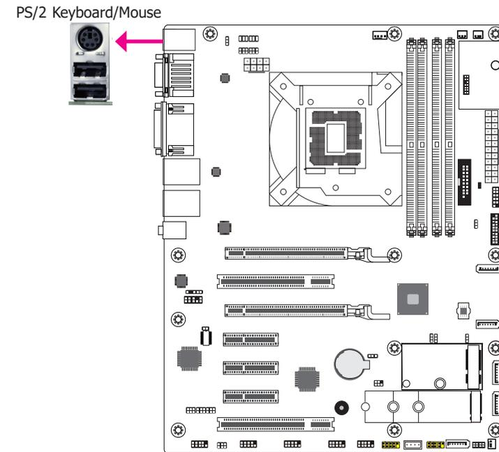
This rear I/O port is used to connect a PS/2 keyboard/mouse. The PS/2 mouse port uses IRQ12.
