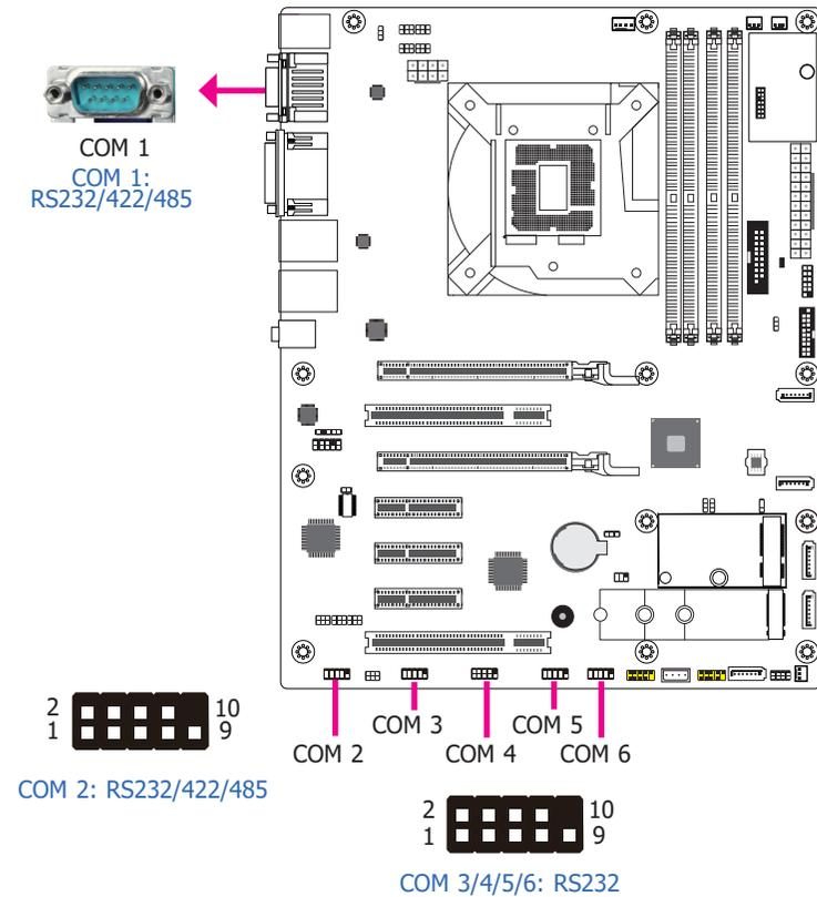
The pin functions of COM 1 port will vary according to setting of JP5, JP6, JP7 and JP8. Refer to "COM1/COM2 RS232/422/485 Select" and "COM1/COM2 RS232/Power Select" in this chapter for more information.
