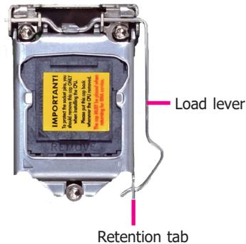
5. Lift the load lever to lift the load plate.
