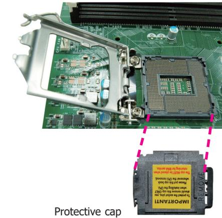
7. Insert the CPU into the socket. The gold triangular mark on the CPU must align with the corner of the CPU socket shown on the photo.
