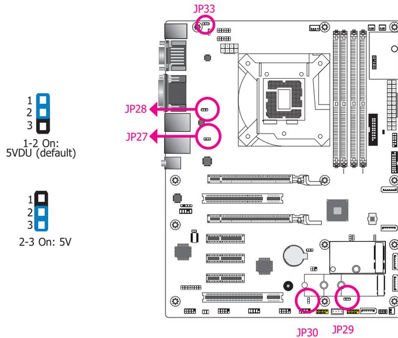
The power of the USB connectors' voltage buses can be configured to either 5V DU or 5V. The jumpers are located as illustrated above and correspond to each USB port number as listed below.
