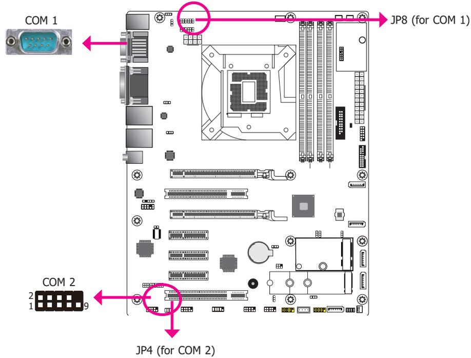
JP8 (for COM 1) and JP4 (for COM 2) are used to configure Serial COM ports to pure RS232 or RS232 with power. The pin functions of COM 1 and COM 2 will vary according to JP8's and JP4's settings respectively.
