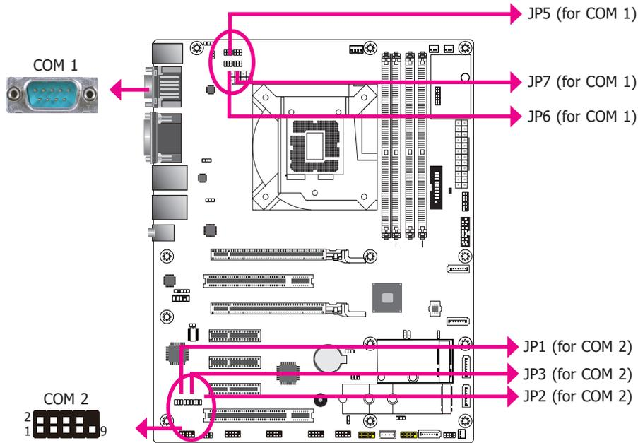
JP5/JP6/JP7 (for COM1) and JP1/JP2/JP3 (for COM2) are used to configure the COM ports to RS232, RS422 (Full Duplex) or RS485. When COM 1 RS232/422/485 is selected, JP6 and JP7 must be set in accordance to JP5. When COM 2 RS232/422/485 is selected, JP2 and JP3 must be set in accordance to JP1. The pin functions of the COM ports will vary according to the jumpers' setting.
