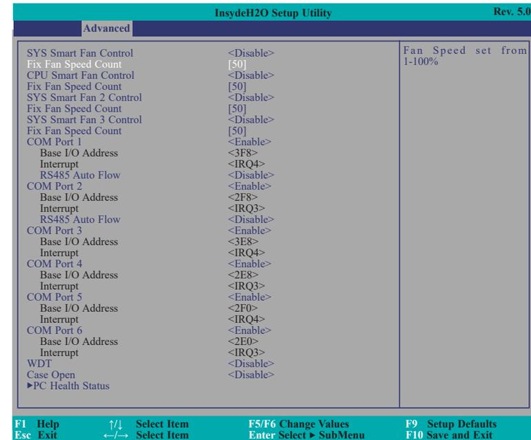
**SYS Smart Fan/Fan 2/Fan 3 and CPU Smart Fan Control**
