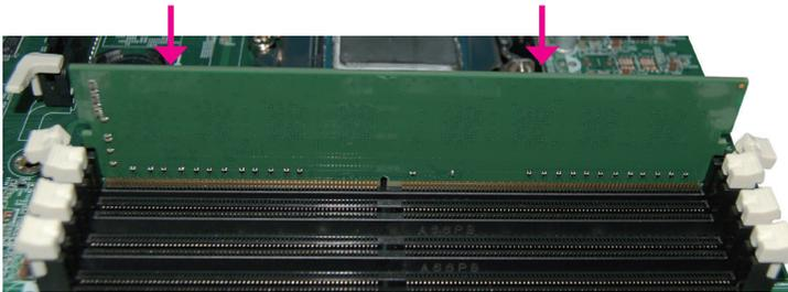
8. The ejector tabs at the ends of the socket will automatically snap into the locked position to hold the module in place.
