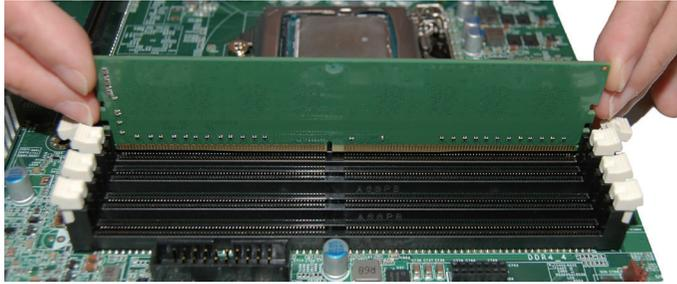
7. Seat the module vertically, pressing it down firmly until it is completely seated in the socket.
