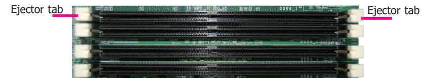
5. Note how the module is keyed to the socket.
