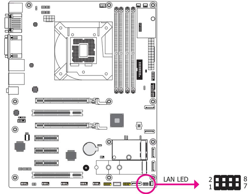
The LAN LED connector is used to detect the connection state of RJ45 LAN ports when the connection is made to an active network via a cable. The pin functions of the LAN LED connector are listed below.
