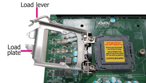
6. Remove the protective cap from the CPU socket. The cap is used to protect the CPU socket against dust and harmful particles. Remove the protective cap only when you are about to install the CPU.
