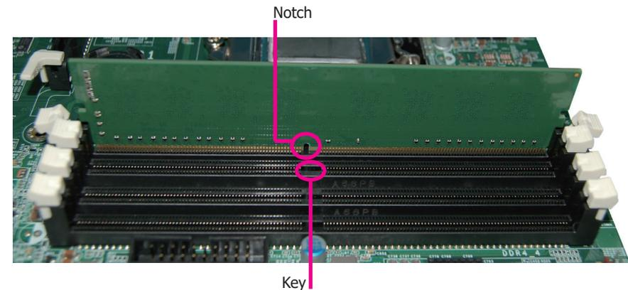
6. Grasping the module by its edges, position the module above the socket with the “notch” in the module aligned with the “key” on the socket. The keying mechanism ensures the module can be plugged into the socket in only one way.
