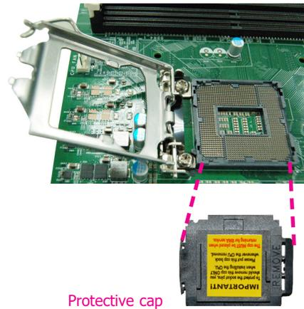
7-1. Insert the CPU into the socket. The gold triangular mark on the CPU must align with the chamfer corner of the CPU socket shown in the photo.
