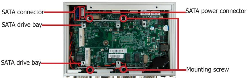
3. Align the mounting holes of a SATA drive with the mounting holes on the drive bay and connect the SATA cable (data and power) to the 2.5" SATA drive. Then, use the provided HDD mounting screws to affix the HDD to the drive bay.
