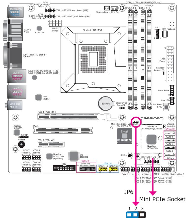
JP6 is used to select the signal for the Mini PCIe socket.
