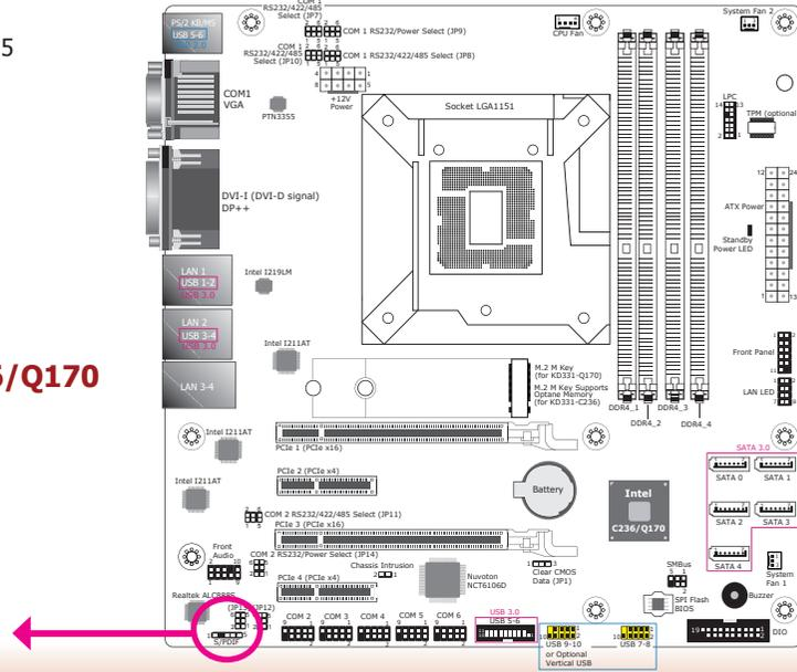
The S/PDIF connector is used to connect an external S/PDIF port. Your S/PDIF port may be mounted on a card-edge bracket. Install the card-edge bracket to an available slot at the rear of the system chassis and connect the audio cable to the S/PDIF connector. Make sure pin 1 of the audio cable is aligned with pin 1 of the S/PDIF connector.
