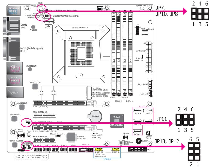
JP7, JP8, and JP10 (for COM1) and JP11, JP12, and JP13 (for COM2) are used to configure the COM ports to RS232, RS422 (full duplex) or RS485. The pin assignments of the COM ports will vary according to the jumpers' settings.
