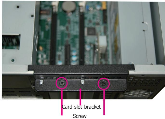
2. Insert the expansion card in the connector on the motherboard and press down until secured.
