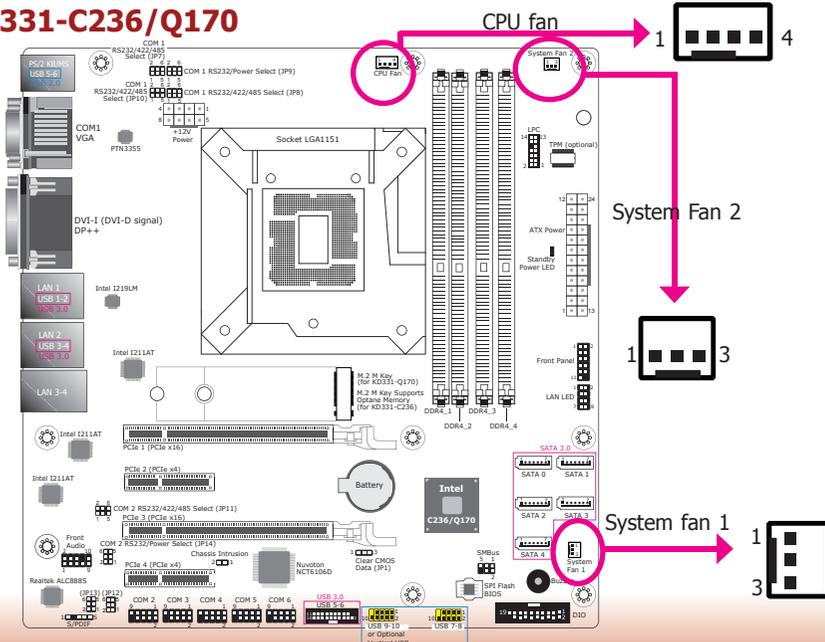
The fan connectors are used to connect cooling fans. The cooling fans will provide adequate airflow throughout the chassis to prevent overheating the CPU and system board components.
