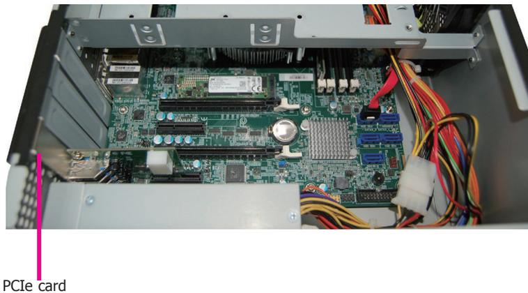
3. Reinstall the card slot bracket to secure the expansion card in place.
