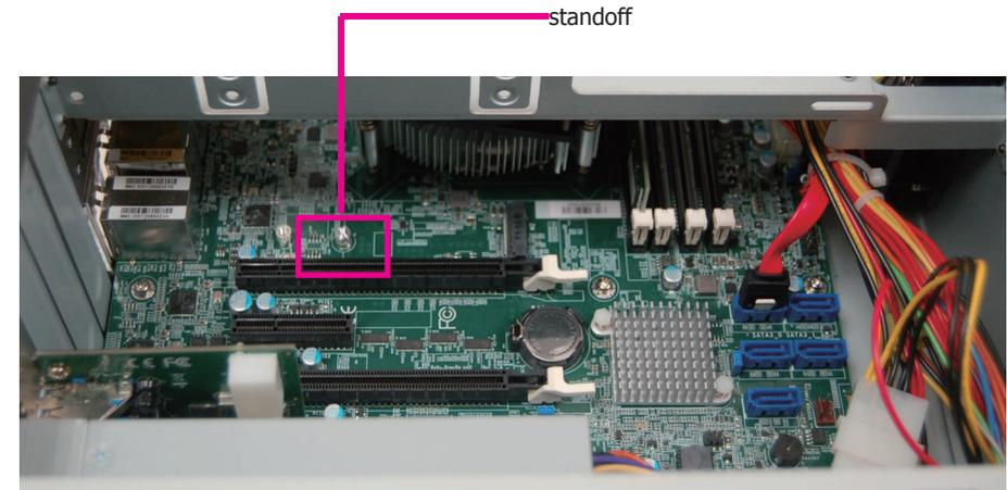
2. Align the notch at the edge of the M.2 card with the key in the connector.
