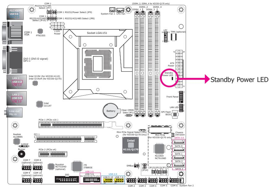
This LED will be red when the system is in the standby mode. It indicates that there is power on the system board. Power off the PC and then unplug the power cord prior to installing any devices. Failure to do so will cause severe damage to the motherboard and components.
