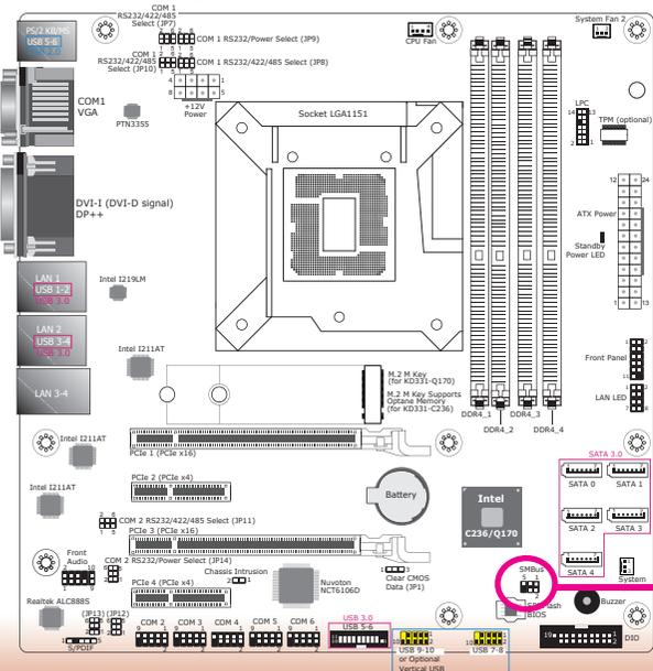
The SMBus (System Management Bus) connector is used to connect SMBus devices. It is a multiple device bus that allows multiple chips to connect to the same bus and enables each one to act as a master by initiating data transfer.
