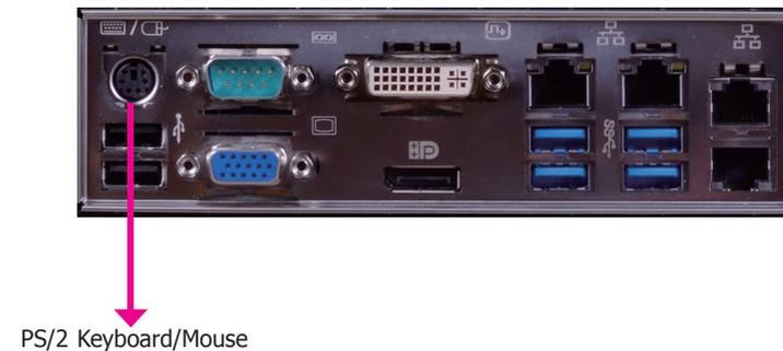
These ports are used to connect a PS/2 mouse/keyboard.
