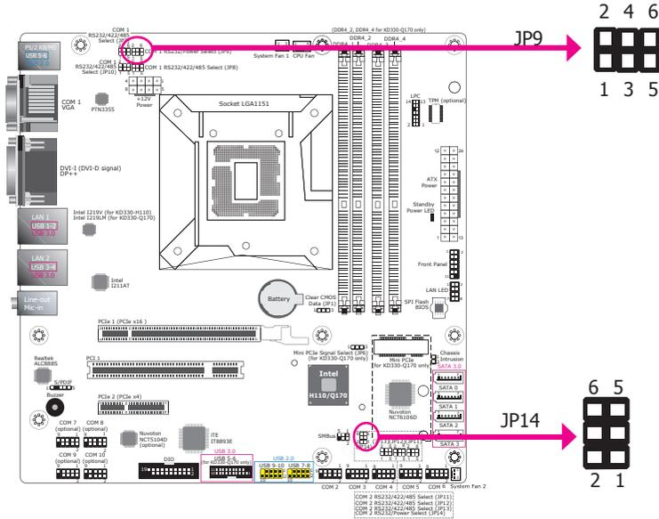
JP9 (for COM1) and JP14 (for COM2) are used to switch the COM ports to RS232 or RS232 with power. The pin assignments of the COM ports will vary according to the jumper settings.
