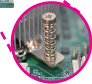
"Unlocked" position of the screw
