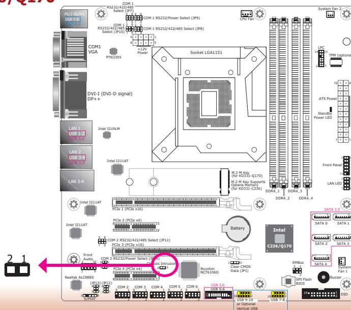
The board supports the chassis intrusion detection function. Connect the chassis intrusion sensor cable from the chassis to this connector. When the system's power is on and a chassis intrusion occurs, an alarm will sound. When the system's power is off and a chassis intrusion occurs, the alarm will sound only when the system restarts.
