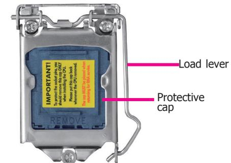
4. Unlock the socket by pushing the load lever down, move it sideways until it is released from the retention tab, and then lift the load lever up.
