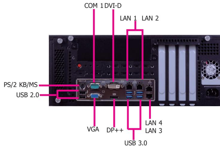
The rear panel I/O consists of the following ports:
