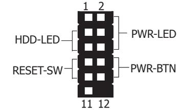
This connector provides several control and LED indicator functions.
