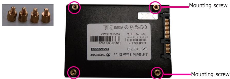
2. Secure the hard drive to the optical drive tray. Align the standoffs on the HDD with the mounting holes on the optical drive tray. Use 4 mounting screws to install the hard drive onto the optical drive tray.
