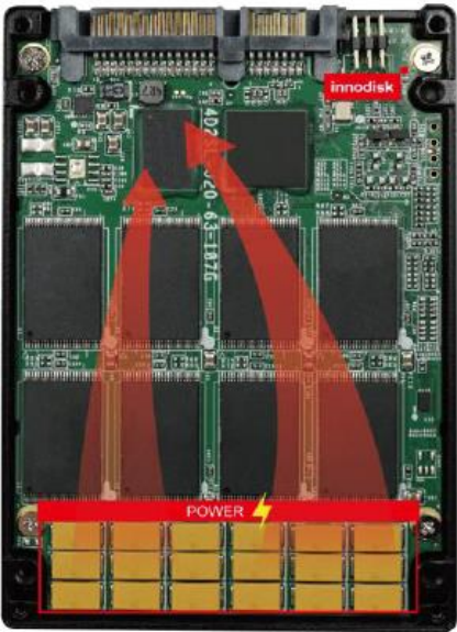
Figure 3: Diagram of 2.5" SATA SSD with iCell
