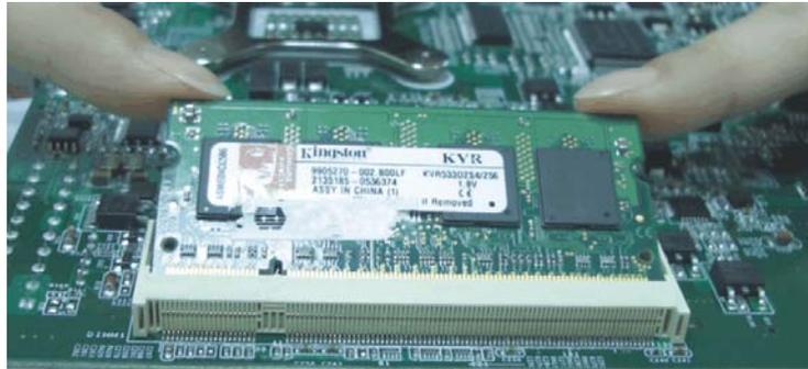
6. Push down the module until the clips at each end of the socket lock into position. You will hear a distinctive "click", indicating the module is correctly locked into position.
