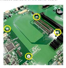
Position the module board on top of the carrier board with its mounting holes aligned with the standoffs on the carrier board and the COM Express connectors of both boards aligned to each other. Press the module board down firmly until it is securely seated on the COM Express connectors of the carrier board.
