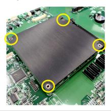
Use the provided mounting screws to secure the heat spreader to the module board and the carrier board.
