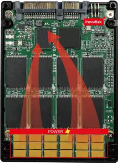
Figure 3: Diagram of 2.5" SATA SSD with iCell
