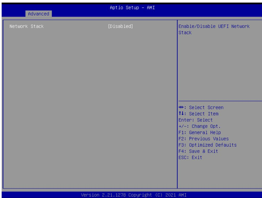
**Figure 3.15 Network Stack Configuration**
