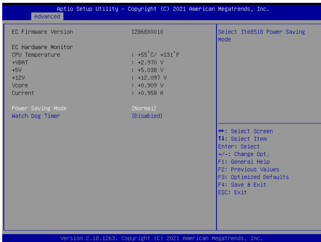
Figure 5.8 Embedded Controller Configuration
