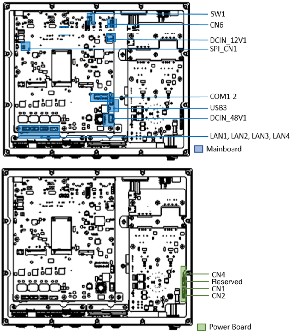
Figure 3.2 Top View of Reserved Connectors
