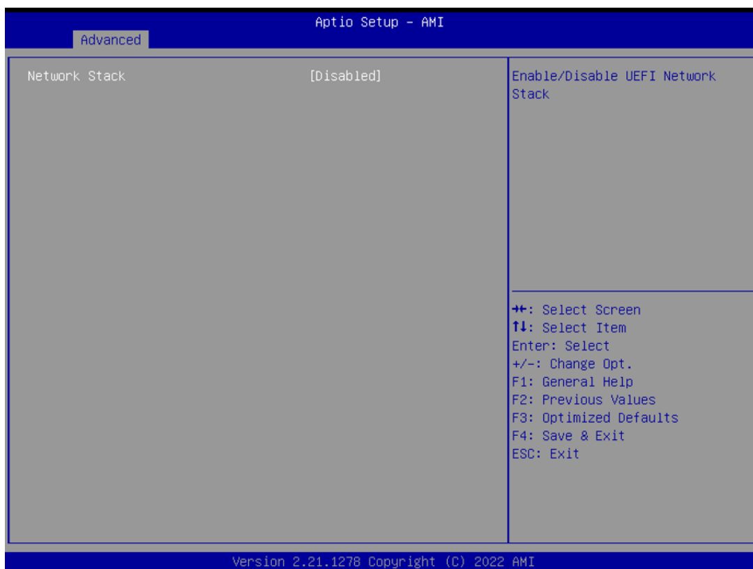
Figure 5.19 Network Stack Configuration
