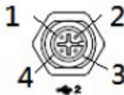
Figure 4.5 USB 2.0 with M12 Connector
