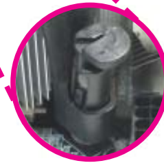
"Unlocked" position of push-pin
