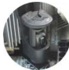
"Locked" position of push-pin
