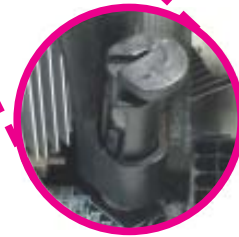
"Unlocked" position of push-pin
