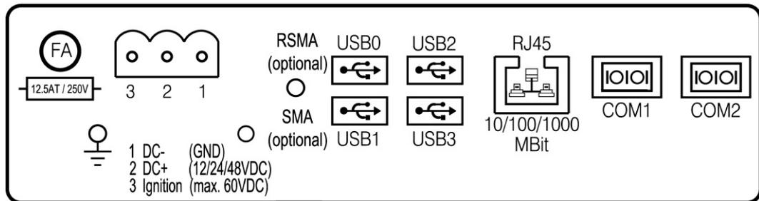
Fig. 13.1: Connectors on the connector panel under the cable cover
