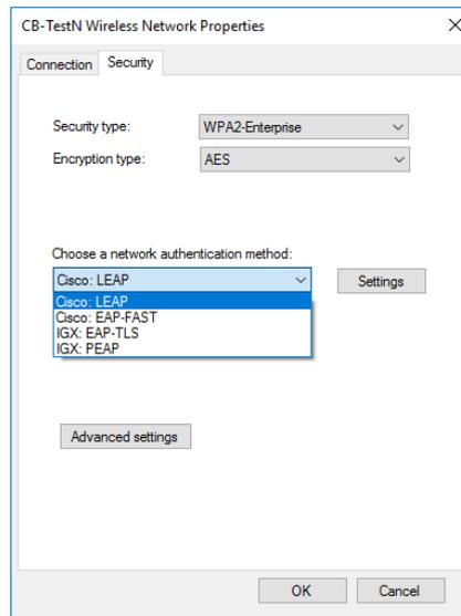
Fig. 10.24: Security settings - network authentication methods
