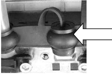
Close off all unused cable openings of the rubber seal using the accompanying blind plugs so that they are sealed.
