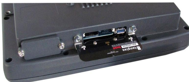
Fig. 7.6: WLAN antenna IEEE 802.11 a/b/g/n/ac opened
