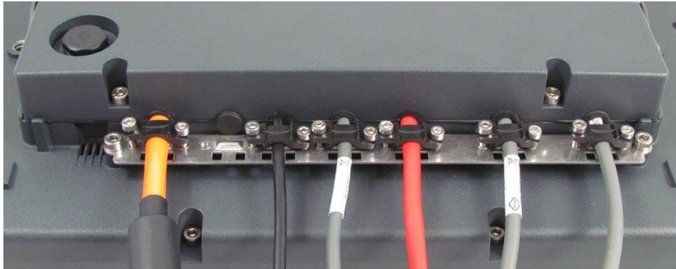
Fig. 13.5: Cable cover closed and screwed together
