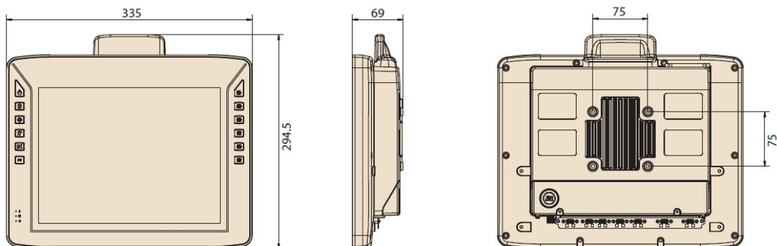
Fig. 5.2: Dimensions DLT-V7212 P, R, D (in mm)
