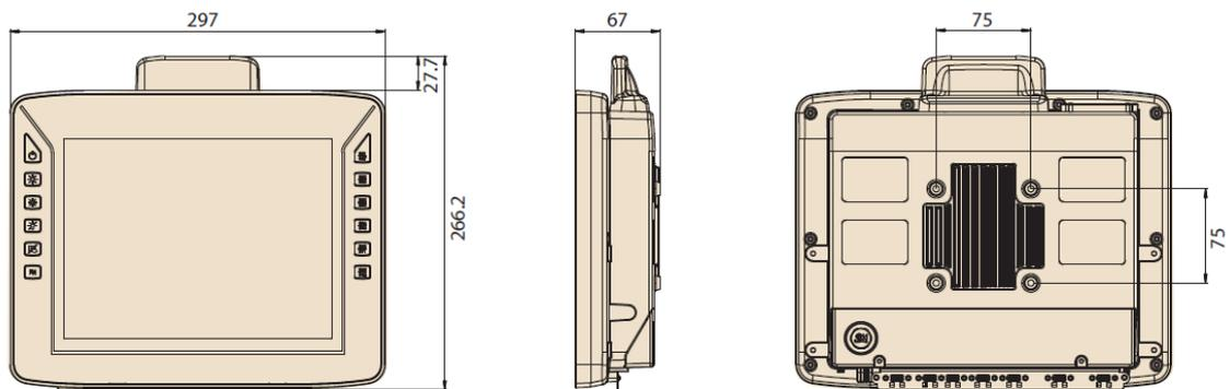
Fig. 5.1: Dimensions DLT-V7210 P, R, D (in mm)
