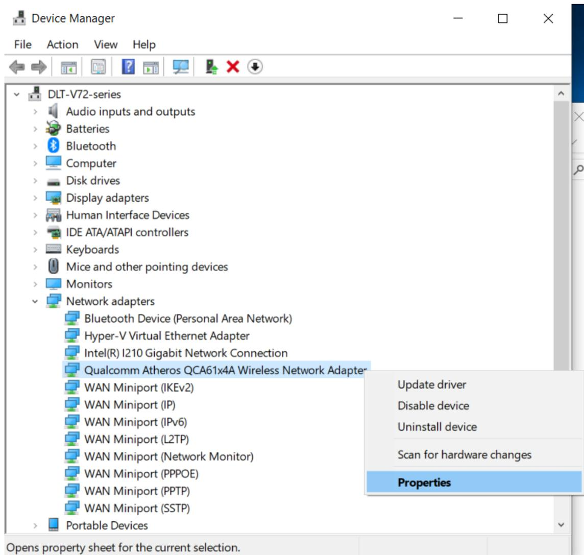
Fig. 10.7: Device Manager network adapter Properties (Qualcomm)
