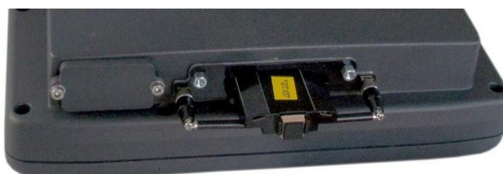
Fig. 7.9: WLAN, WWAN LTE 4G antenna opened
