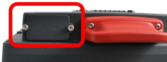
Fig. 14.1: Battery pocket with UPS DLT-V72
