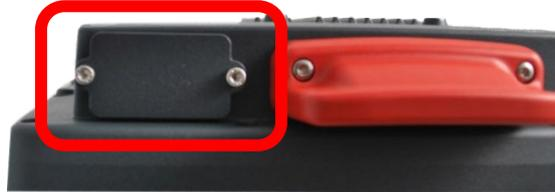
Fig. 8.5: Battery pocket with UPS DLT-V72
