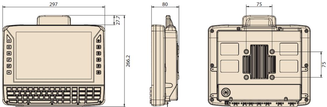
Fig. 5.3: Dimensions DLT-V7210 K, KD (in mm)
