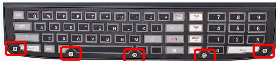
Fig. 16.1: Integrated keyboard: Unscrew the mounting screws
