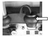
Close off all unused cable openings of the rubber seal using the accompanying blind plugs so that they are sealed.
