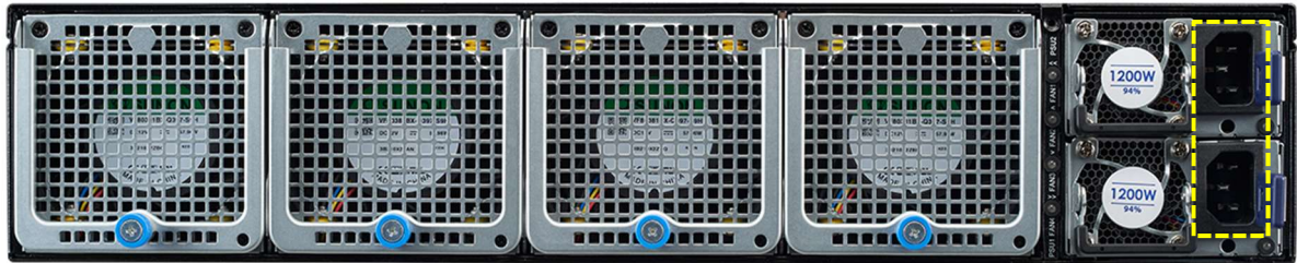
Figure 2.4-12 Location of the Power Inputs
