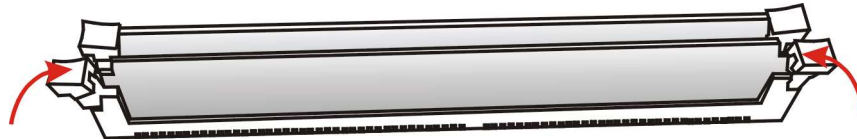
Figure 3.2-9 Seating the DIMM in the Socket
