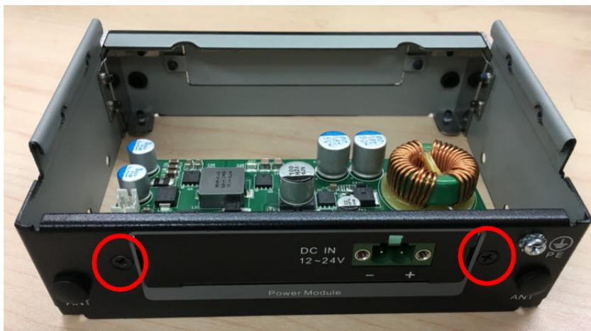
3. Remove the four screws on both sides of ARK-1124.
