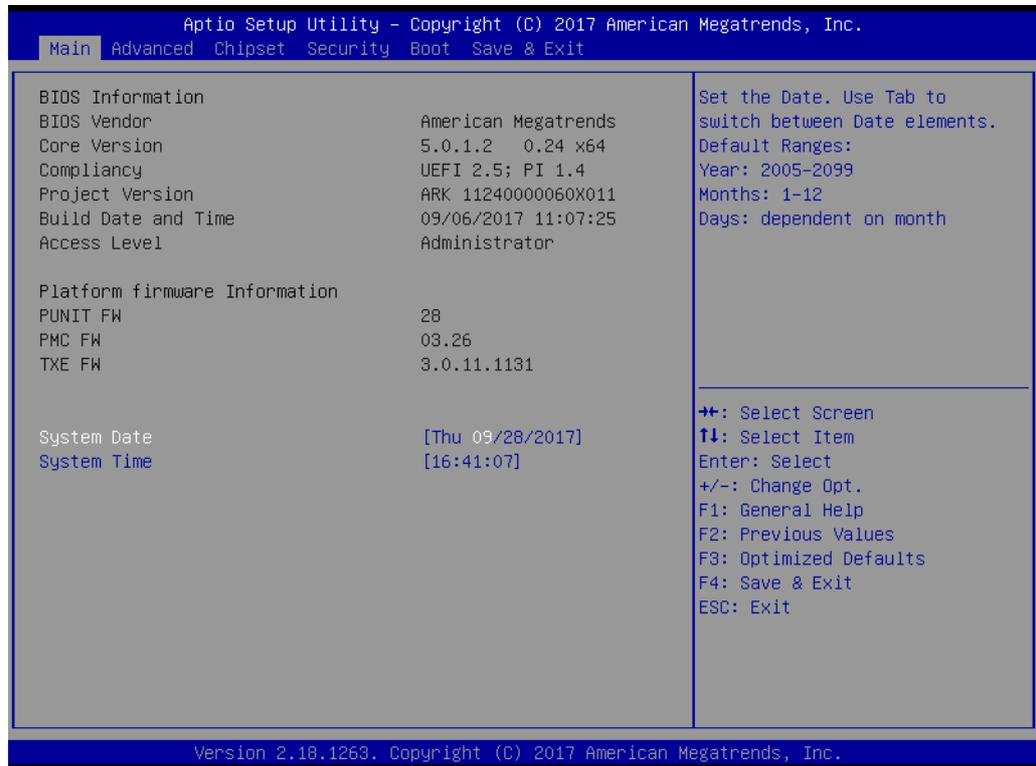
**Figure 3.1 Setup program initial screen**
