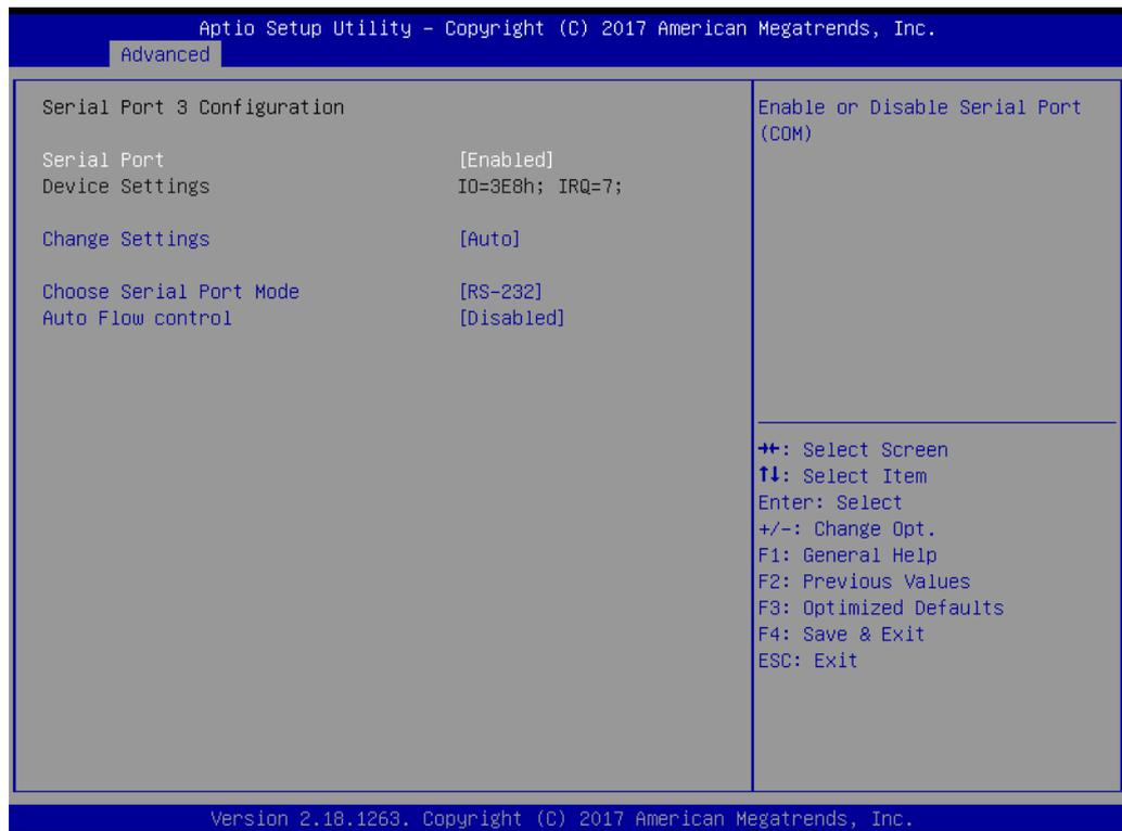
**Figure 3.8 Serial Port Settings (Port3)**
