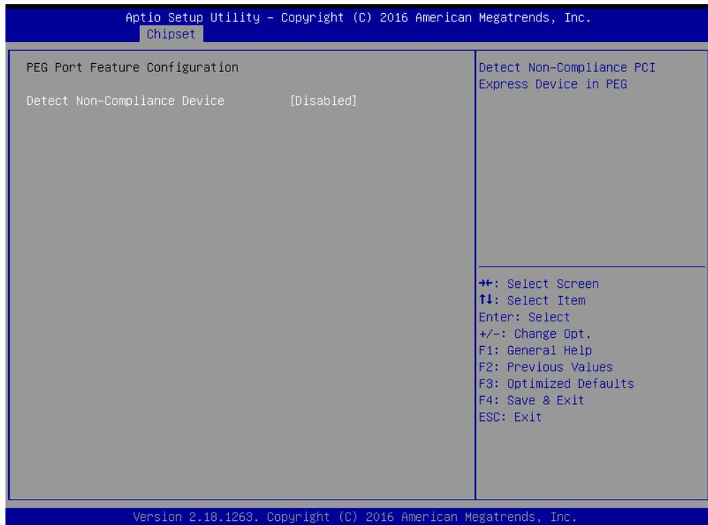
Figure 3.43 PEG Port Feature Configuration
