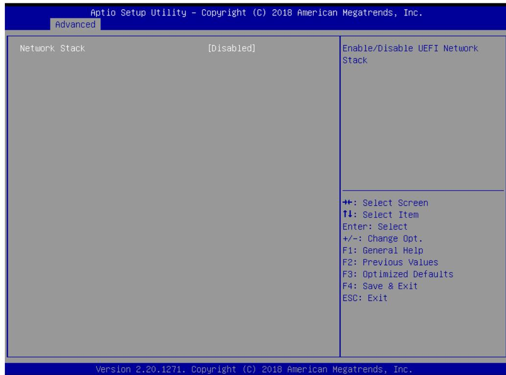
**Figure 3.35 Network Stack Configuration**
