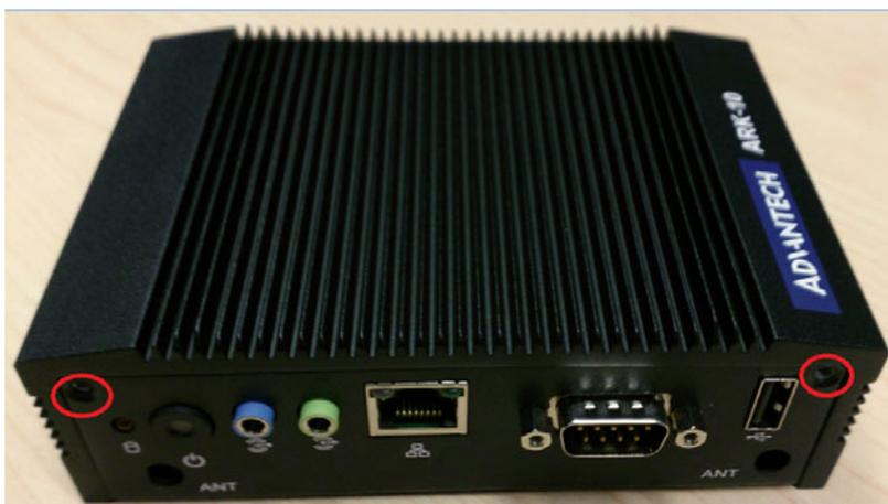
4. Remove aluminum top chassis and install RAM.
