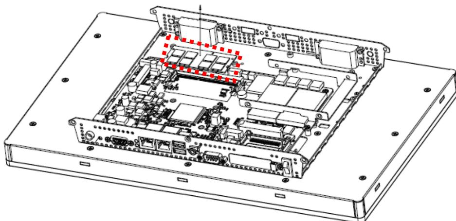
**Step4.** Remove the SODIMM from the memory socket.
