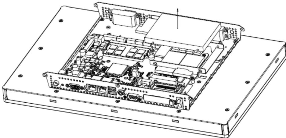
**Step3.** Unfasten 4 screws of the HDD bracket and take it off.
