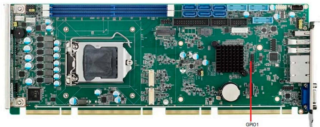
Provides 10-pin header connector for 8-bit Digital I/O usage. Refer to Appendix B for detailed information on the pin assignments and programming guide in Appendix C.
