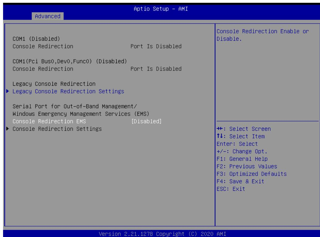
Figure 3.38 Serial Port1 Console Redirection
