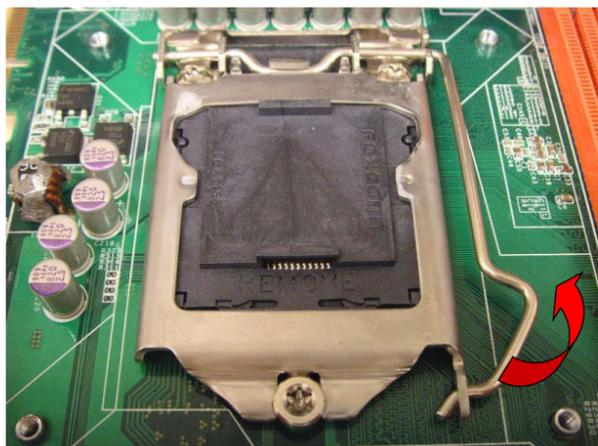
2. Remove the socket protection cap.
