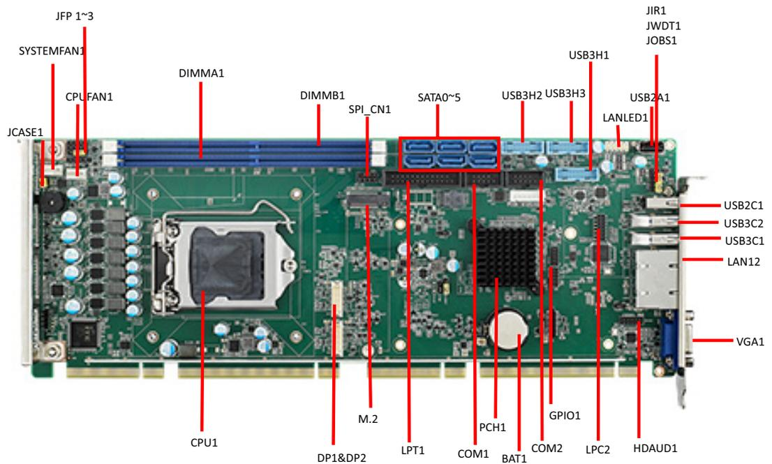
**Figure 1.1 Jumper and Connector Locations**
