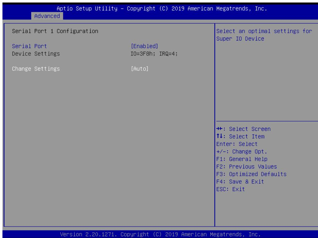
**Figure 3.28 Serial Port 1 Configuration**
