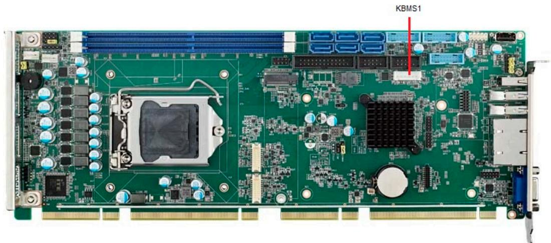
The on-board KBMS1 pin header provides connection to the front panel PS/2 keyboard and mouse connector of the chassis.
