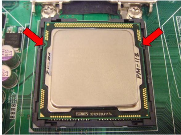
4. Replace the socket cap; lower the retainer bar and clip it shut.
