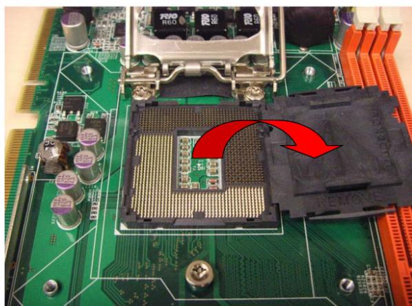
3. Align the cuts on the processor with the edges of the socket.
