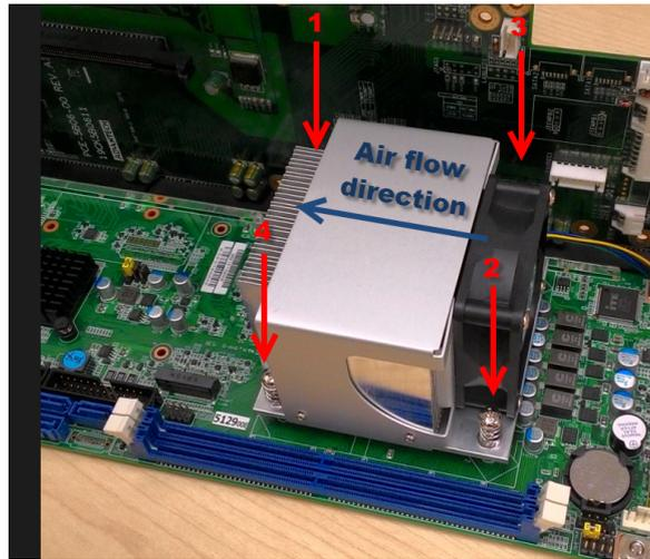
Note the direction of CPU cooler; it must follow that shown above. Installing a CPU cooler in the wrong direction may cause poor heat dissipation that may damage the CPU card.
