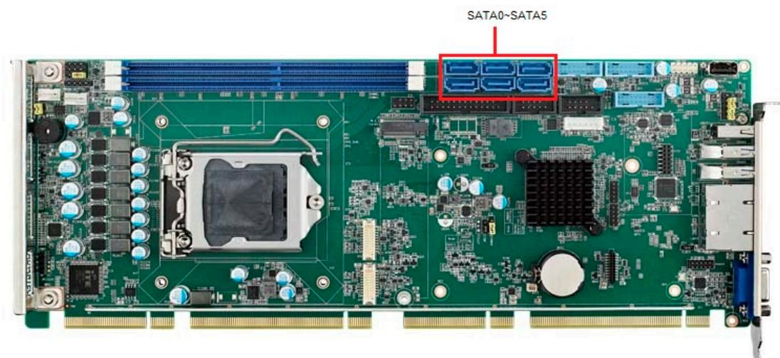
The PCE-7132/5132/5032 features high performance serial ATA interface (5\*600MB/s) which eases cabling to hard drivers or CD/DVD drivers with long cables. These five on-board SATA ports can be configured as RAID 0, 1, 10, or 5 (PCE-5132 do not support RAID). Please see the detailed BIOS setting instructions for this in Chapter 3.
