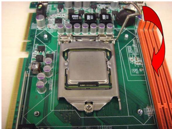
5. The finished processor installation.
