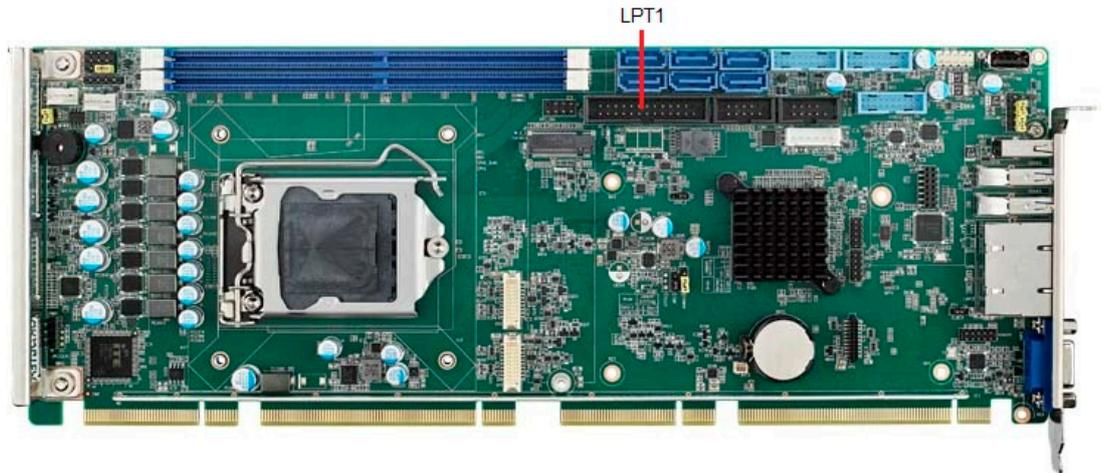
The parallel port is normally used to connect the motherboard to a printer. The SBC includes an onboard parallel port, accessed through a 26-pin flat-cable connector.
