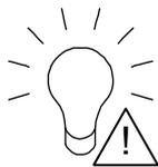
**Power failure:** When this LED flashes, a failure in the power supply is indicated.
