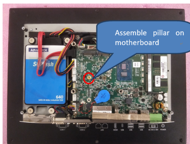
Figure 2.12 Assemble Pillar on Motherboard
