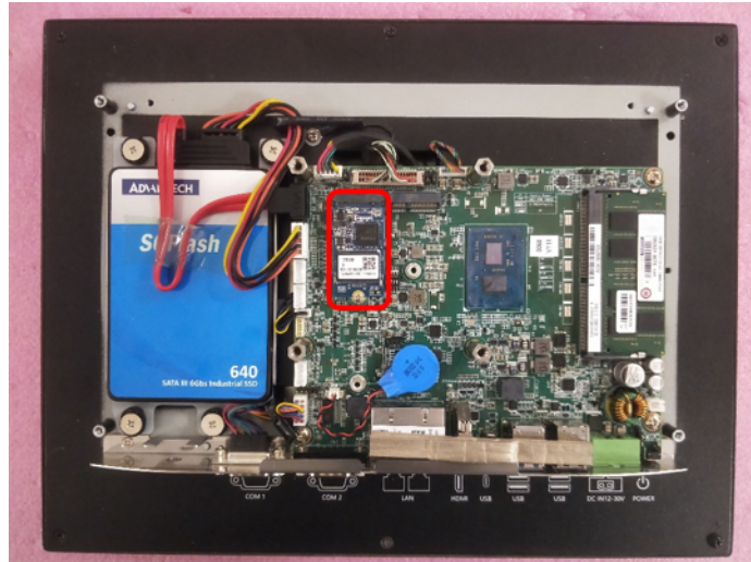
Figure 2.13 Assemble Pillar on Motherboard
