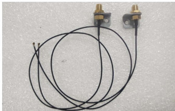
Figure 2.15 Assemble Bracket with Antenna Cable
