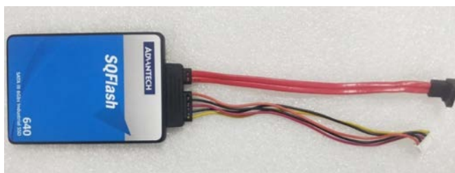
Figure 2.9 SATA Cable Connected to the SATA SSD
