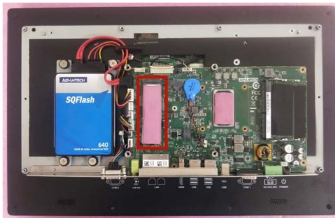
Figure 2.13 Affix the Thermal Pad to the M.2
