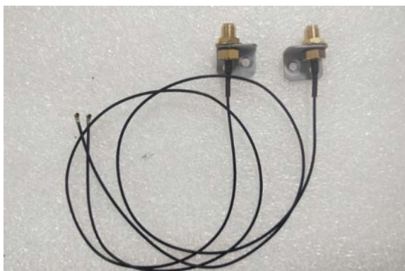
Figure 2.14 Assemble the Brackets to the Antenna Cables
