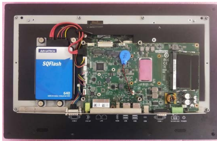
Figure 2.11 SATA SSD Connected to the Motherboard
