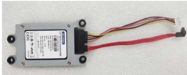
Figure 2.10 Secure the SATA SSD with Screws
