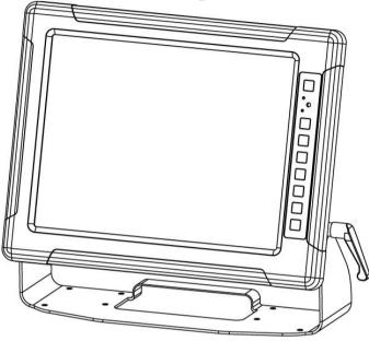
2. Secure three M5x10 screws to fix the device upon the bracket stand.
