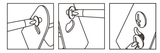
3. Secure tightly locking handle to the Panel PC.
