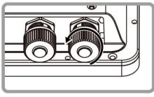
2. Connect power cable to the connector of your device. Make sure the cable fits to the connector, then tighten the O-ring (by turning clockwise) to secure the connection.
