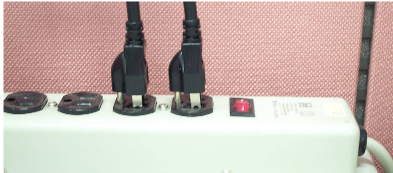
Figure 3.11 Power Cord Plugs Should Have Same Orientation in the Socket/ 插座上电源线方向相同 / 插座上的电源线方向應相同
