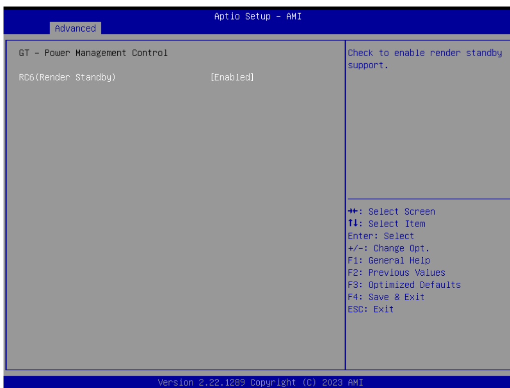
Figure 3.8 GT - Power Management Control
