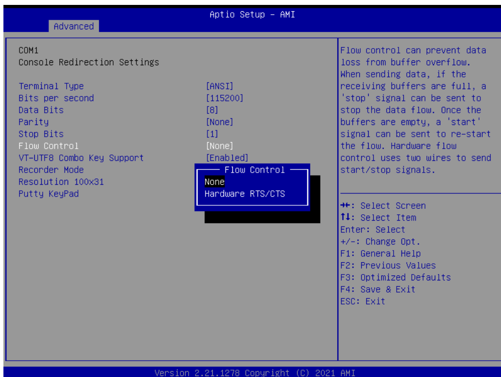
Figure 3.26 Flow Control Settings
