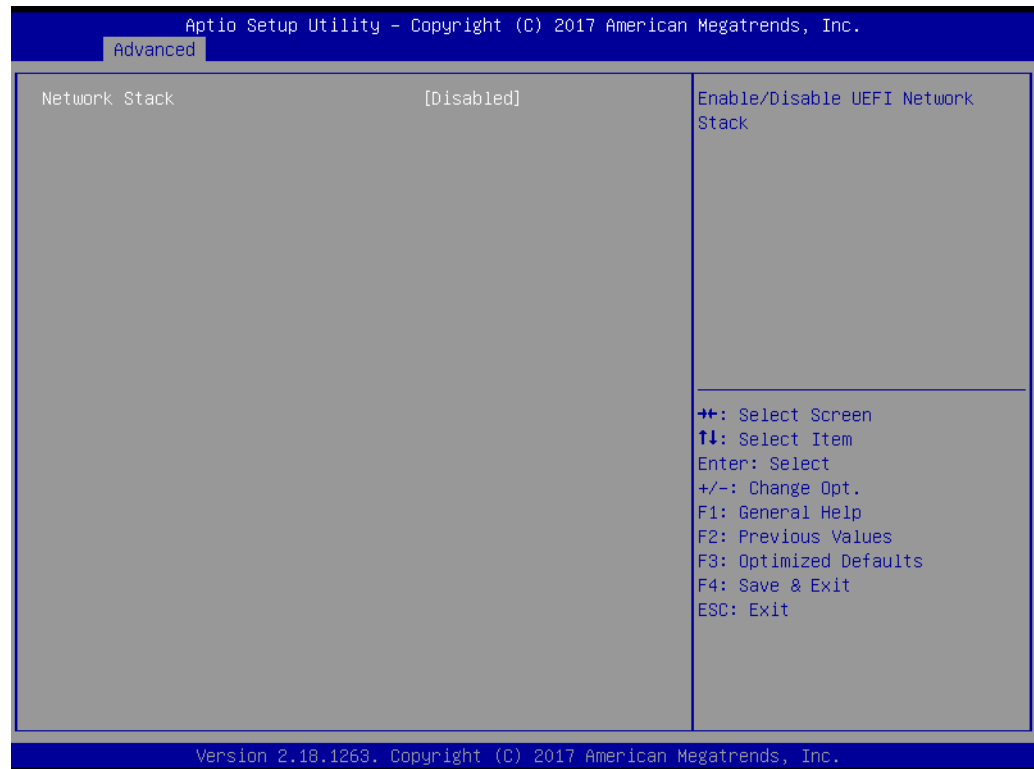
Figure 3.21 Network Stack Configuration
