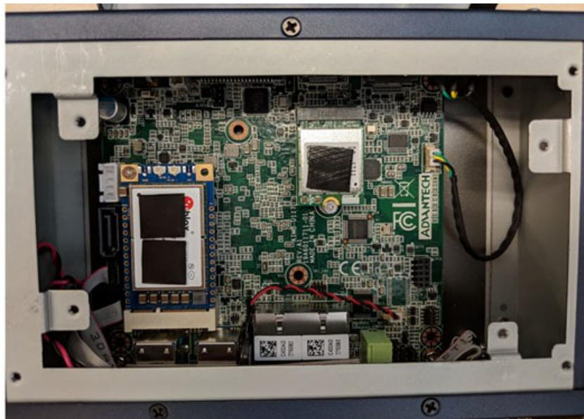
3. Install thermal pad and antenna
