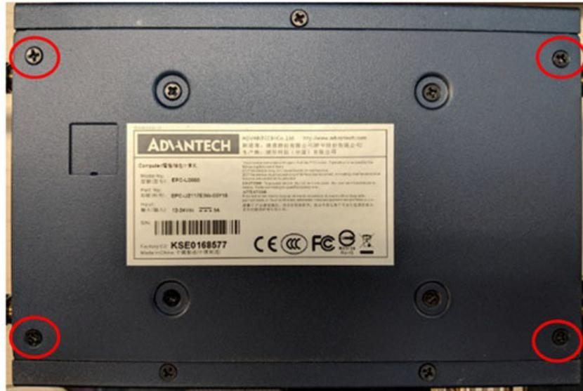
2. Install MiniPCIe module and secure by screw.
